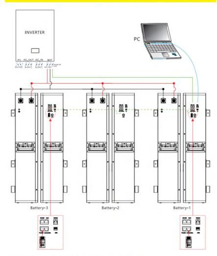
NOTE: The powerlines between each battery are the same length.
